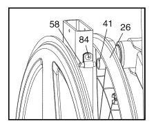
(84). Slide the Reed Switch slightly closer to or away from the Magnet, and then retighten the Screw. Rock the Left Pedal Disc forward and backward just enough that the Magnet passes the Reed Switch repeatedly. Repeat until the console displays correct feedback. When the Reed Switch is correctly adjusted, reattach the shields. Note: If you have questions as to which screw should be in which hole, see EXPLODED DRAWING B on page 27 and the PART LIST on page 24.
